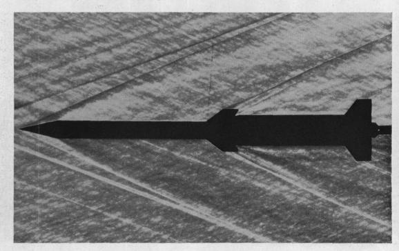
BRIEF ENCOUNTER-A test unit is photographed as it meets a concrete target in a test to determine effects of impact. Individual frames were taken from 70mm color movie film.
